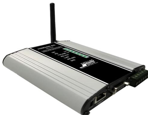
HSM240E-SD, the Swiss knife of modems, provides the added benefit of local control and monitoring and can work with Ethernet, serial, and digital I/O simultaneously. Besides this flexibility, the modem also supports standard Wi-Fi communication with selectable RF speeds up to 54Mbps in standard mode and 108Mbps in turbo mode for point-to-point and point-to-multipoint communication.
