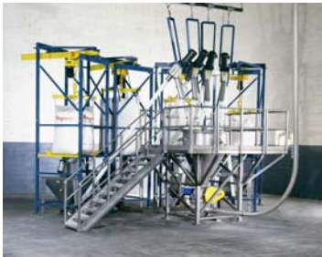
Multiple Bulk Bag Weigh Batching System from Flexicon
